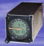
Flight Log Download "Security Fail" - Check security seal in the logger First thing to check when having problems downloading secure flight logs Press knob 10 times (not too fast) to get to screen 10 (screen shows "0") Rotate knob one click to the left Should show "GOOD SEAL" on 302 display Seal status also shown at power-up on 303 display
